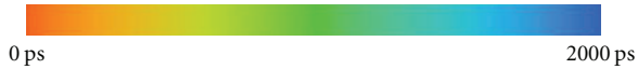
FIGURE 3: A false-colour scale, in this case corresponding to 0–2000 ps, is used to define the fluorescence lifetime decay rate of each fluorophore: for each colour, there is a corresponding value of lifetime decay.
