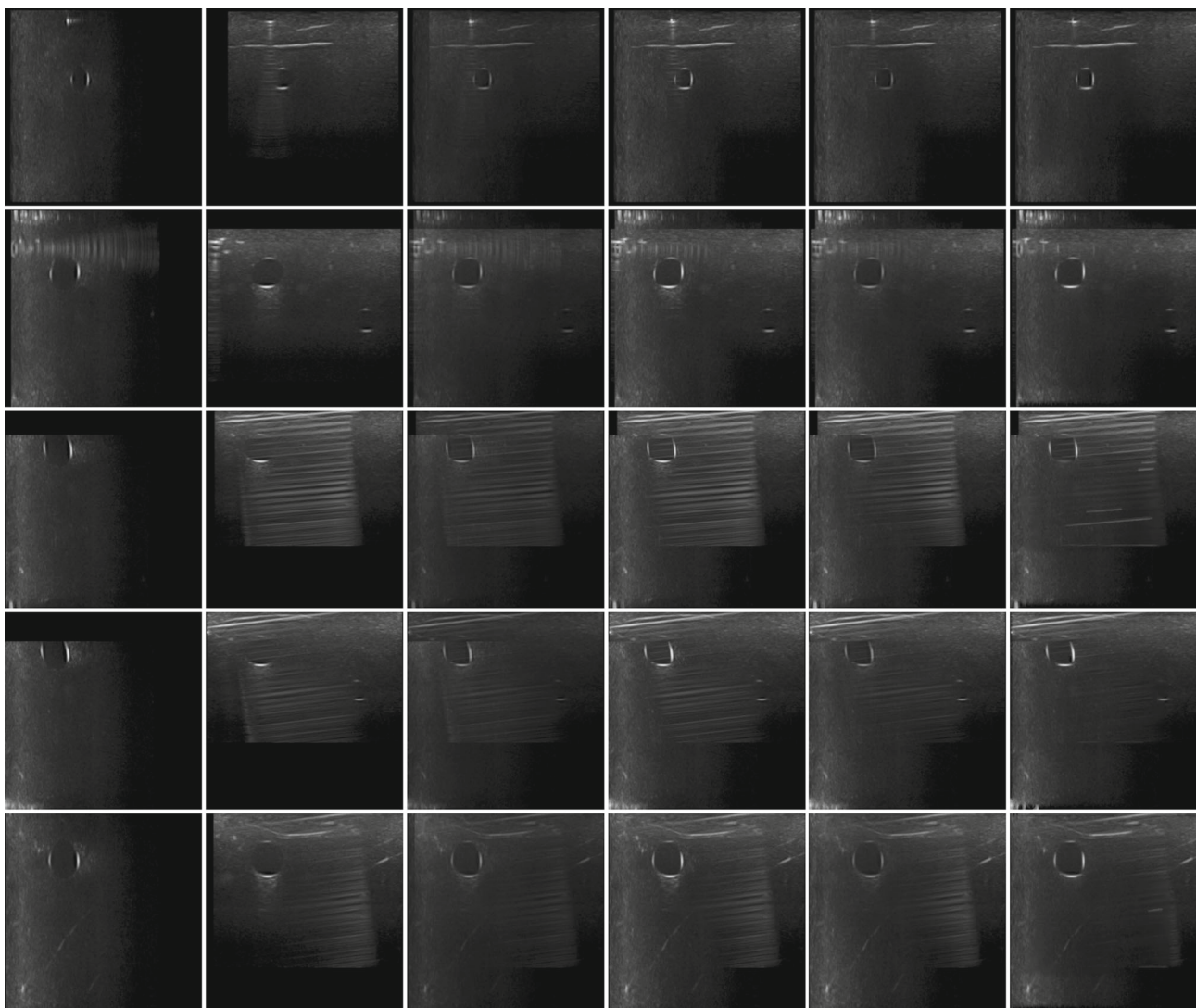
Fig. 5 Results on the phantom with a needle inserted in it. The left two columns are the two input images. (Phantom images were acquired orthogonally within plane, where the imaging direction of the first and second column is from left to right and from top to bottom, respectively.)
