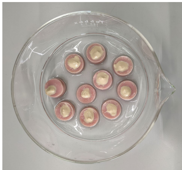
Fig. 1 Bovine teeth with NMTD treatment placed in the container with artificial saliva on the bottom prior to sealing
