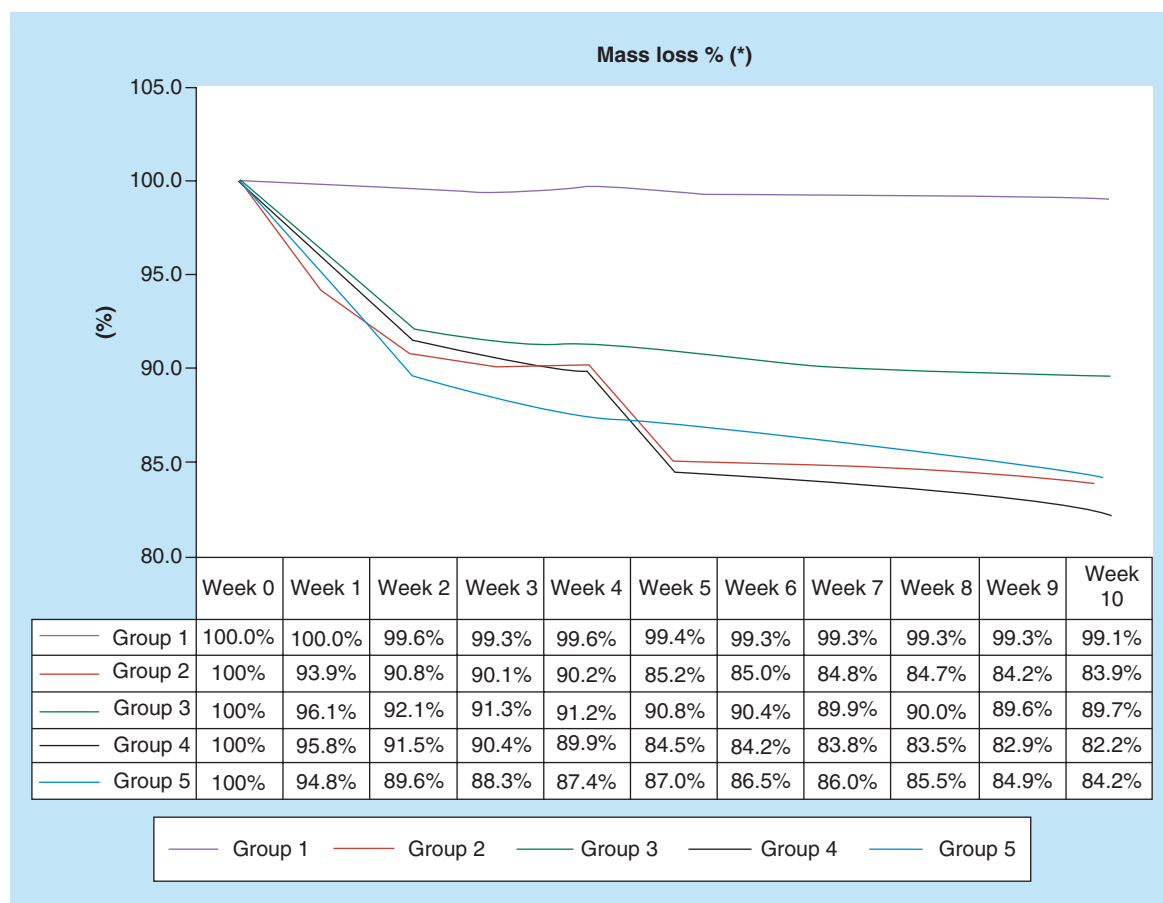
Figure 3. Mass loss delta%. All experimental groups have had mass loss during 10 weeks. On the experimental groups, the group 2 and 4 had more mass loss and both were under sodium hypochlorite solution.
