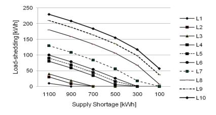
In the CEL application, as shown in Figure 8, equal load-shedding is applied to load agents not limited by their power claims and amounts of load claims are imposed to load agents limited by their
