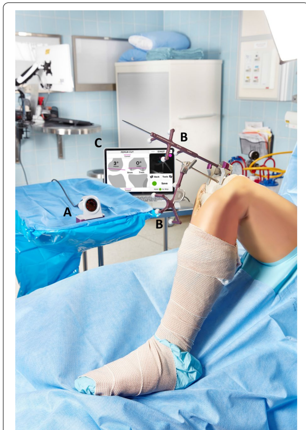
Fig. 1 During use, the camera (A) detects movement of the trackers (B) within its field of view and relays information to the computer workstation (C), which sits outside of the sterile field. The workstation displays intraoperative data in real time and is controlled by the surgeon using buttons on the camera or by an assistant using the keyboard
