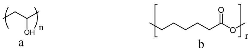
Figure 3. Chemical structures of synthetic polymers (a) poly (vinyl alcohol) and (b) poly ( \epsilon -caprolactone).
