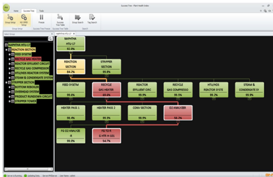
Figure 14. Success tree for the Hydrotreating unit.
