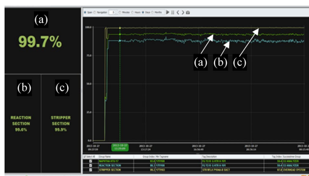
Figure 12. Example display of the PHI indicating the (a) overall plant health index and the health indices of the (b) reaction and (c) stripper sections.
