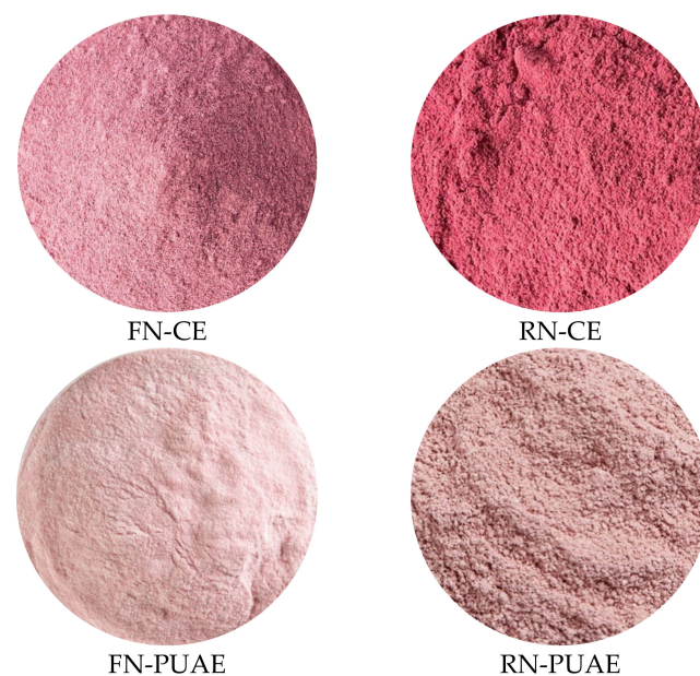
Figure 5. Images of pectin samples extracted from Fetească Neagră (FN) and Rară Neagră (RN) grape pomace by conventional extraction (CE) and pulsed ultrasound-assisted extraction (PUAE).
