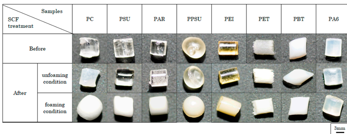
Figure 3. Appearance of pellets formed using different engineering plastics before and after supercritical treatment.
