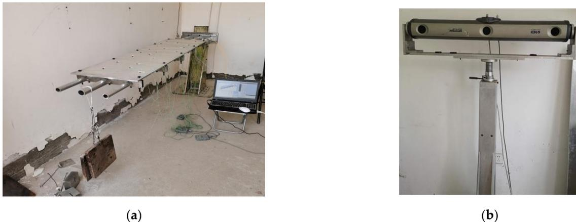
**Figure 13.** Experimental platform: (a) Loading on end-node of entire structure; (b) NDI Optotrak Certus.
