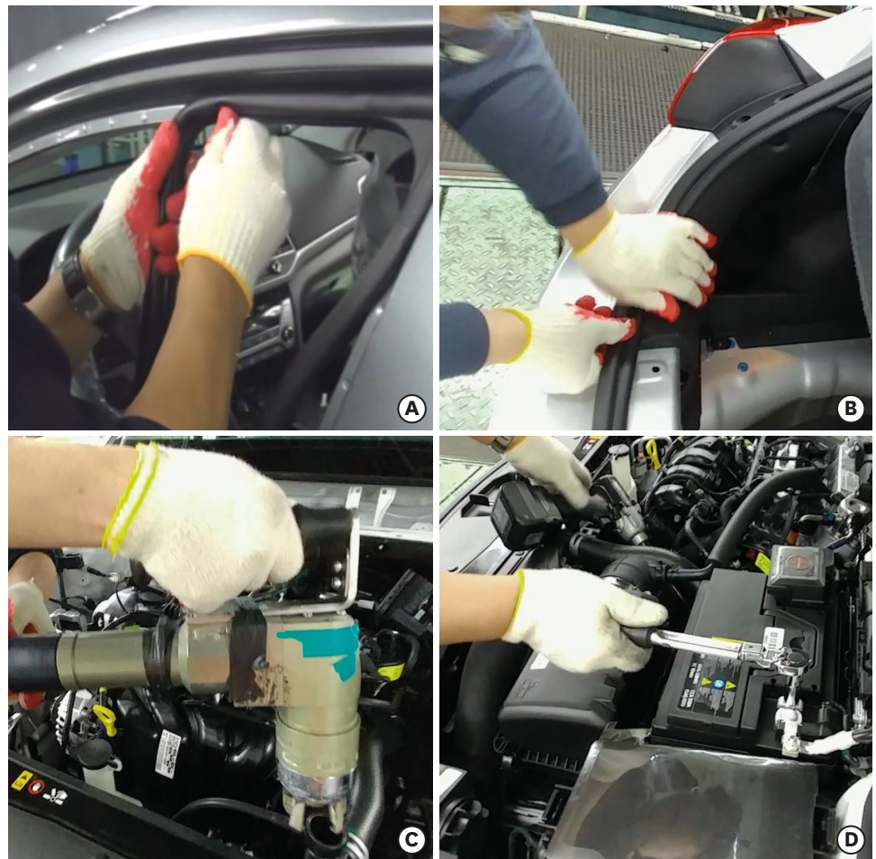
Fig. 3. Thumb and wrist joints burden of the patient's tasks. Extension of the thumb and ulnar deviation of the wrist are thought to be burden on the extensor pollicis longus tendon. (A, B) Extension of the thumb: applying pressure while installing door trim and trunk garnish (C) Ulnar deviation of the wrist: holding the hand-arm vibration tool while injecting antifreeze liquid (D) Repetitive motion of the wrist: tightening a screw with the wrench while installing air cleaner, battery cable, and duct.
