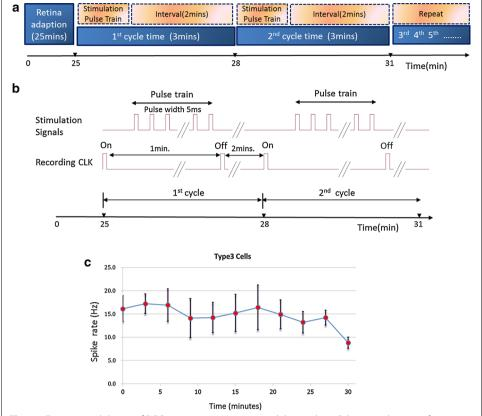
**Fig. 10** Experimental design of RGC response against time and the results. **a** Schematic diagram of experimental design. **b** Stimulations were delivered every 3 min with 1 min pulse train and 2 min interval. Stimulation signals and time clock control (CLK) of recording signals are indicated. **c** The spike rate of a type III RGC during recording. The first 25 min was the habitation period
