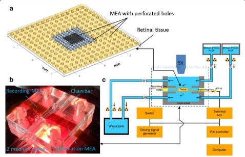
Fig. 8 Illustration of MTM platform. **a** The perfusion holes in the MEA surface. In the center (*gray*), middle (*blue*) and outer (*yellow*) regions of the MEA, the diameters of diffusion holes were 10, 50 and 100 μm with 10, 20 and 20 % OAR, respectively. **b** The acrylic perfusion chamber under the microscope. **c** The experimental setup of MTM platform. The perfusion system and the directions of the fluid flow are labeled
