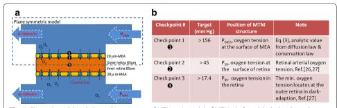
**Fig. 2** Physical model and physical parameters of MTM. **a** A model of MTM platform labeled with predetermined parameters and the positions of three checks points. The perfusion paths could improve oxygen transfer rate and also create negative fluidic pressure to properly put retina tissue on MEAs with minimum gaps. **b** The required  $PO_2$  in the three check points are listed
