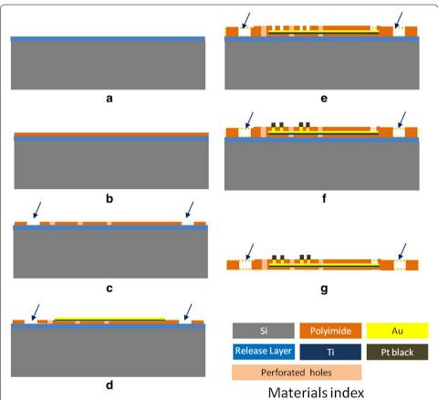
**Fig. 3** The fabrication process of perforated MEA: **a** substrate with release layer deposited; **b** first polyimide spin coating; **c** polyimide patterning and curing; **d** Metal layer (Au and Ti) deposition and patterning; **e** second polyimide coating, patterning and curing; **f** Au and Pt black electroplating; **g** physically detach the device from the substrate. *Arrows* indicate the diffusion holes
