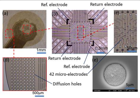
**Fig. 7** Optical microscope picture of the MEA device. **a** Picture of the head of the MEA. **b** Enlarged picture of the head of the MEA. **c** The central region of the MEA, note the microelectrodes and diffusion holes. **d** The outer region of the MEA. **e** SEM photo of the microelectrode (×5000). The diameter is about 11.5 µm
