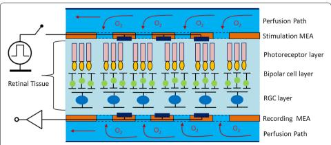
**Fig. 1** An ideal MEA-Tissue-MEA (MTM) platform. It illustrates the perfusion paths of oxygenized fluid, stimulation MEA, recording MEA and retina tissue. Both stimulation and recording MEAs have porous holes to improve the oxygen diffusion rate
