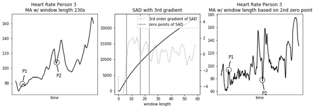
Fig. 9. Heart rate, sum of absolute differences with third gradient, and heart rate with moving average filter with window length based on second zero-point of third gradient, for Person 3 from PAMAP2 dataset.
