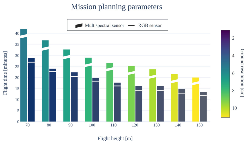
Fig. 5. Mission planning parameters compared with different visual sensors.
