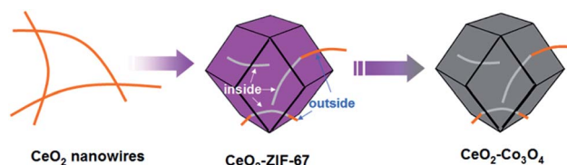
Fig. 1 The synthetic steps of short \text{CeO}_2 nanowires inserted porous \text{Co}_3\text{O}_4 nanoframeworks.
