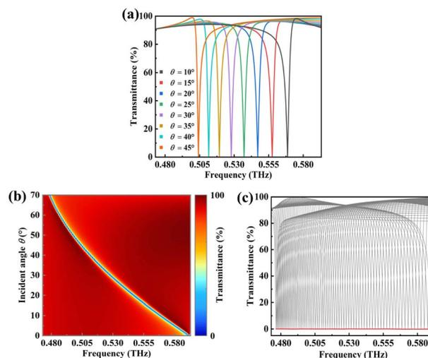
Fig. 4 (a) Transmittance spectra of the metasurface for various incident angles. (b) A two-dimensional contour map of transmittance as a function of the incident angle ( $1^\circ$  to  $70^\circ$ ) and frequency. (c) Transmittance spectra (incident angle ranging from  $1^\circ$  to  $70^\circ$ ) and the corresponding envelope curve of the metasurface.
