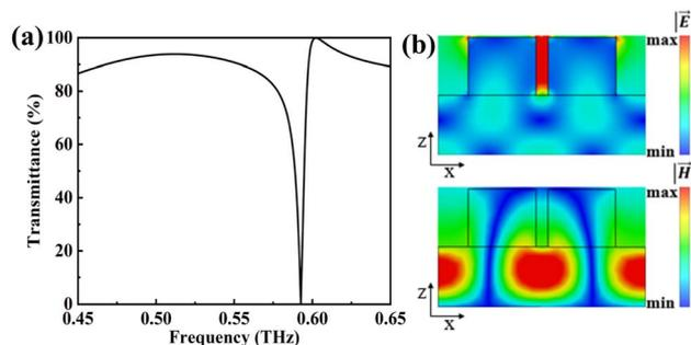
Fig. 2 (a) Transmittance spectrum of the proposed metasurface ranging from 0.45 to 0.65 THz. (b) Absolute value distribution of the electric field (top) and magnetic field (bottom) in the  $x$ - $z$  plane of the metasurface at the resonance.
