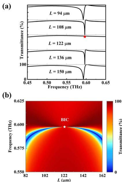
Fig. 3 (a) Transmittance spectra of the metasurface with different  $L$  values. The red pentagram is the accidental BIC. (b) Two-dimensional diagram of transmittance as a function of frequency and parameter  $L$ . The white pentagram is the accidental BIC.
