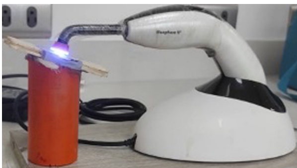
Fig. 2: Device designed to ensure a 1 mm distance during polymerization.
