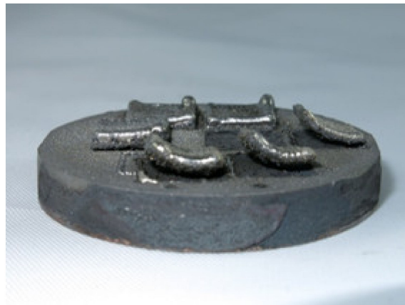
Figure 6. Fe6Al LENS®samples on a sintered Fe-Al substrate.
