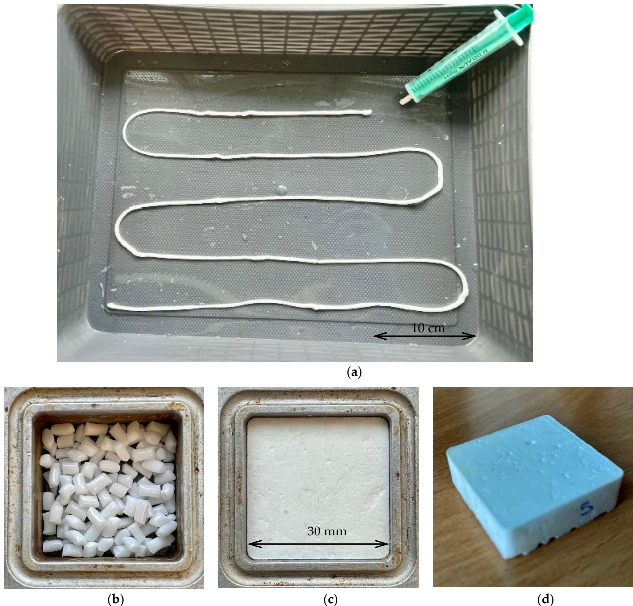
Figure 2. (a) Expandable epoxy extrudate with a diameter of 2.7–3.5 mm and a length of 1.5 m, (b) EEBs in mold, (c) EPF after foaming at 160 °C and cooling and (d) EPF after demolding.
