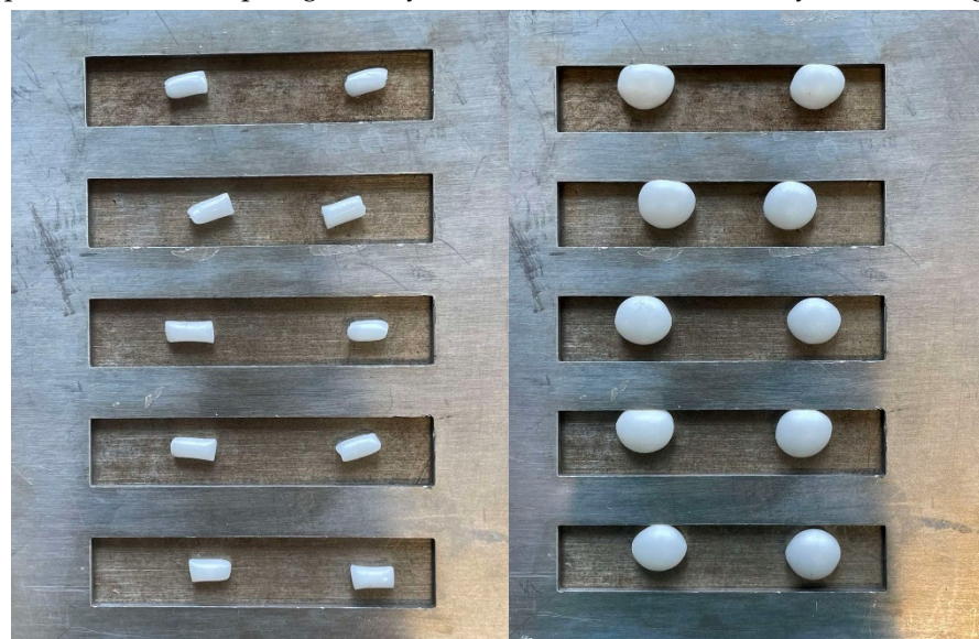
Figure 6. Tan-3 EEBs (left) and their expanded epoxy beads after foaming at 150 °C (right).
