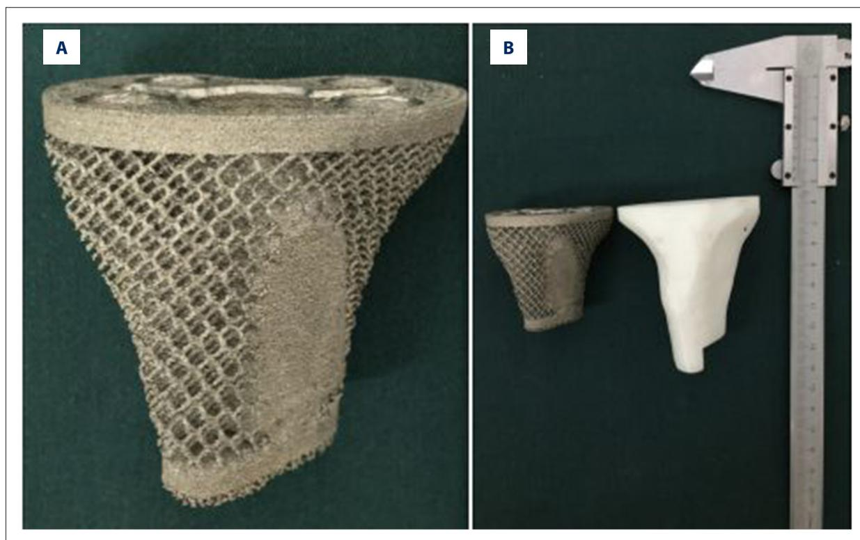
**Figure 6.** The final product made of titanium alloy. (A) The reticular porous structure on the surface. (B) Comparing with model made of photosensitive resin.
