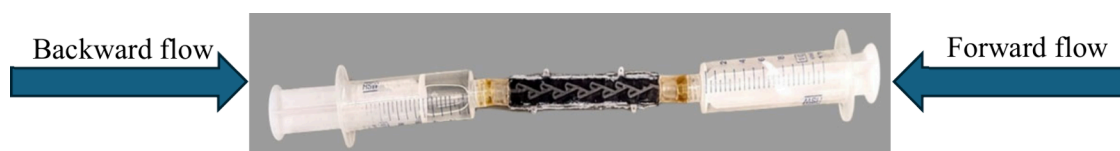
Figure 1. Nanobubble generation by flow regime switching using a Tesla valve.
