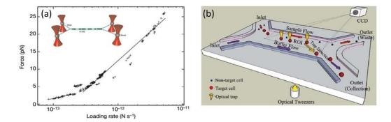
**Figure 1.** (a) Inset: Scheme of  $\lambda$ -DNA molecules linked by H-NS suspended between polystyrene beads held with optical tweezers; Dynamic force spectrum of the H-NS–DNA interaction. The two distinct regions in the Spectrum are fitted to straight lines. (Reprinted with permission from Springer Nature [50]); and, (b) Scheme of a lab-on-a-chip sorting procedure with optical tweezers (Reproduced from [51] with permission of the Royal Society of Chemistry).
