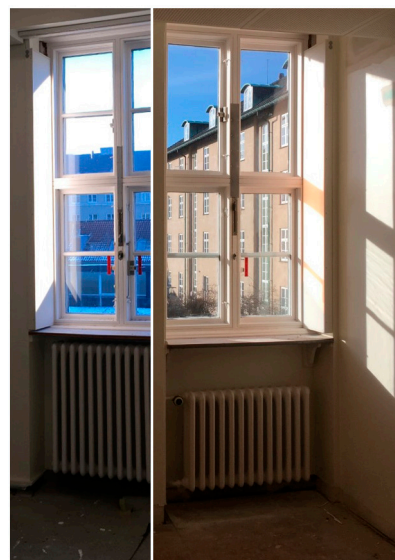
Figure 1 The left-hand picture shows how the light-emitting diode panel is mimicking sunlight reflections on the wall. The right-hand side of the picture shows natural sunlight reflexions on the wall.
