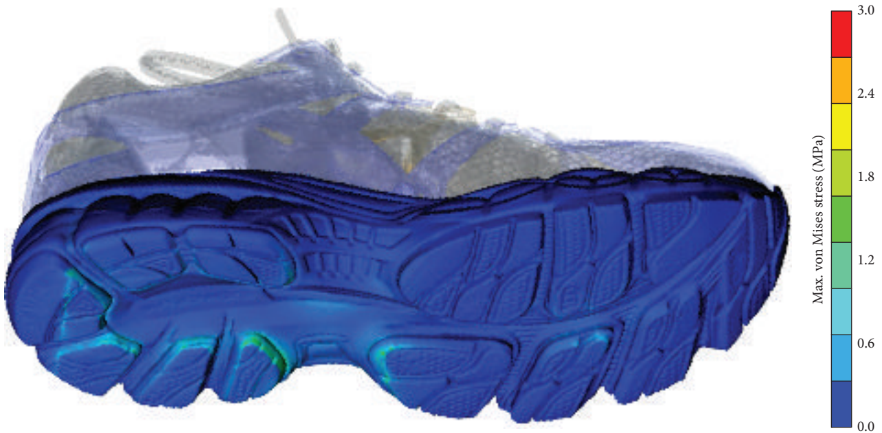
FIGURE 6: Equivalent von Mises stress distribution during an intermediate step of impact peak.
