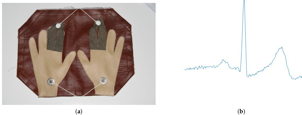
Figure 2. Example of the device and the ECG from the CYBHi dataset. (a) Example of the device used to get the ECG signal. Source: [20]. (b) Example of the ECG shape extracted from the CYBHi dataset.
