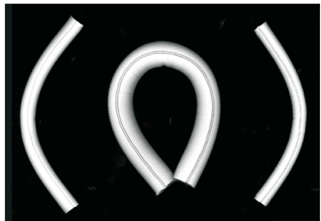
Fig. 1. The test vascular polyester polyethylene terephthalate (PET) graft with internal diameter ranging from 8-30 mm.
