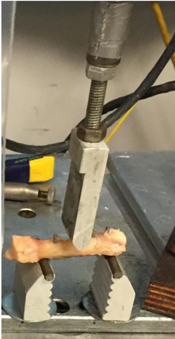
Fig. 4 Testing setup with loading pin centered over osteotomy producing an apex dorsal force on the MTS servohydraulic frame
