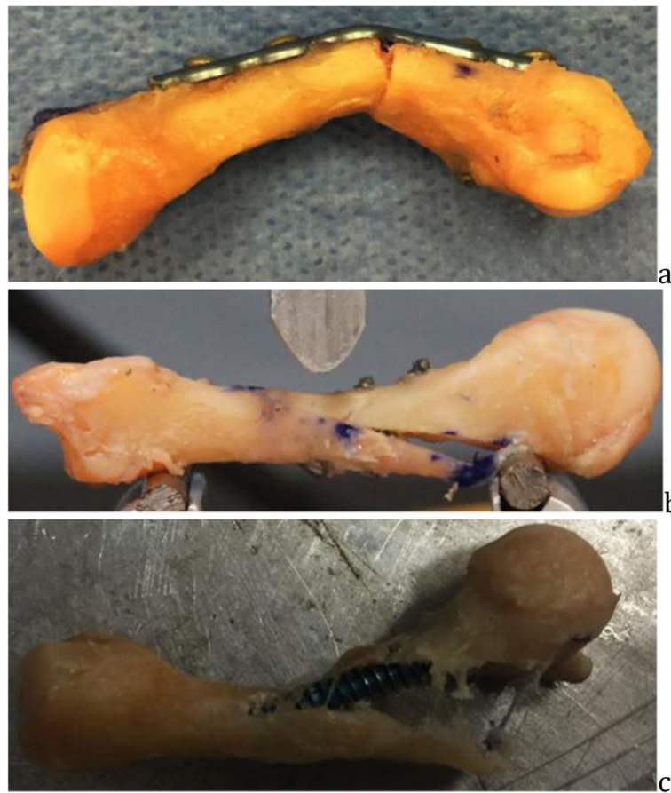
Fig. 5 Failure patterns, a plate bending in a transverse osteotomy, b lag screw disengagement in oblique osteotomy, and c headless compression screw loosening in metacarpal head and displacement at osteotomy site of oblique pattern
