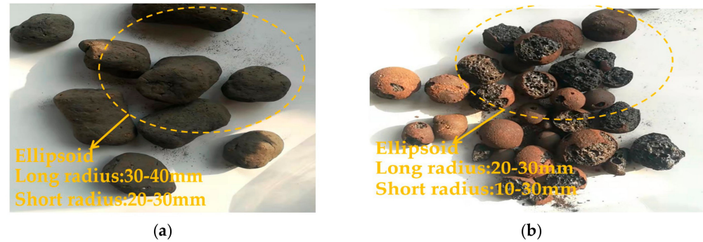
Figure 1. Photos of sludge ceramsite and clay ceramsite. (a) Sludge ceramsite. (b) Clay ceramsite.
