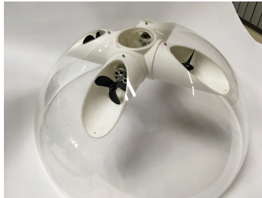
Figure 3. Final placement of the manifolds in a hemisphere of the prototype UV.
