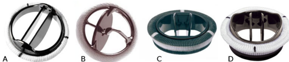
Fig. 1 The four types of mechanical aortic valves used. The St Jude (a) and the Medtronic Hall (b) valve are pictured from below and the Carbomedics (c) and ON-X (d) valve are pictured from above. Note the variable position of the leaflet hinge points. The hinge points are below the level of the housing ring in the St Jude valve (a) and are at the level of the housing ring in the Carbomedics (c) and ON-X (d)
