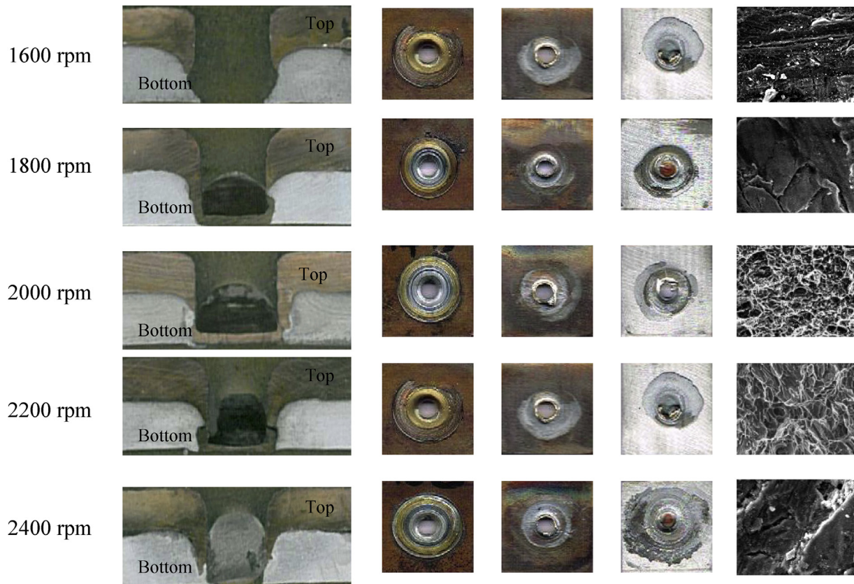
Figure 5. Effect of rotational speed on cross-section of weld, top side of top sheet, bottom side of top sheet, top side of bottom sheet and fracture surface.
