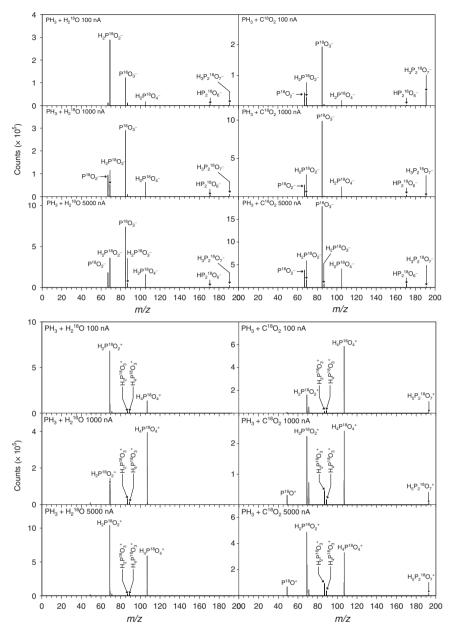
**Fig. 2** SIMS data from residues of irradiated phosphine-doped ices. The spectra were recorded in the negative (top) and positive ion mode (bottom) correlated with the formation of <sup>18</sup>O-substituted oxoacids formed in irradiated phosphine (PH<sub>3</sub>)-water (H<sub>2</sub><sup>18</sup>O) (right) and phosphine (PH<sub>3</sub>)-carbon dioxide (C<sup>18</sup>O<sub>2</sub>) (left) ices
