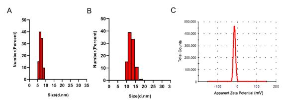
**Figure 3.** Characterization of PD-L1 aptamers and Apt-HJ by dynamic light scattering (DLS). (**A**) Size distributions of free PD-L1 aptamers. (**B**) Size distribution of Apt-HJ. (**C**) Zeta potential distribution of Apt-HJ.
