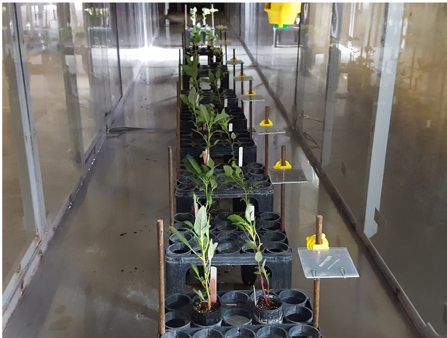
Fig 2. Herbicide particle drift study conducted in the low speed wind tunnel with waterhemp ( Amaranthus tuberculatus ), Palmer amaranth ( Amaranthus palmeri ), and drift collectors (Mylar cards) positioned at different downwind distances from the nozzle.
