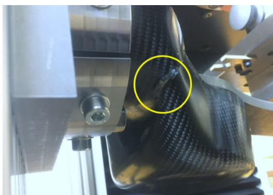
Failure at the limb neck due to compression
