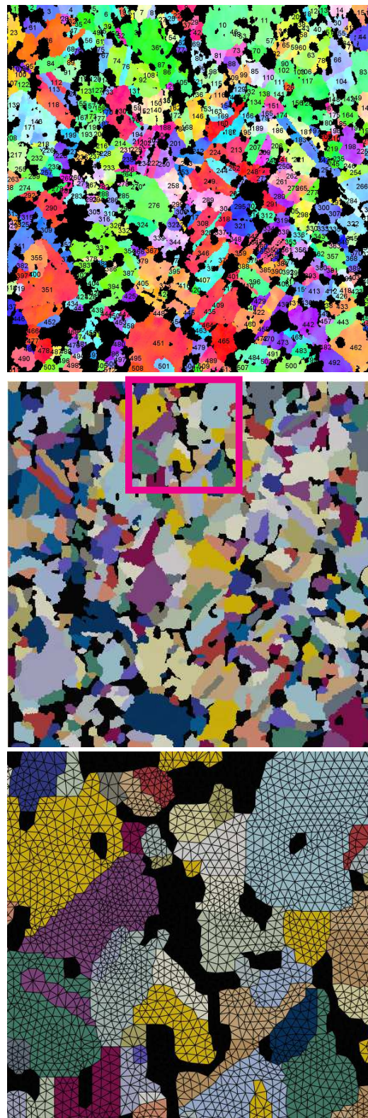
Figure 6. The real microstructure of Figure 2a with 513 Ag grains ( upper ); after pixel selection ( middle ); selected-region meshing ( lower ).
