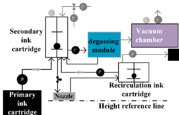
Fig. 9. Ink supply system schematic diagram.
