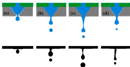
**Fig. 8.** Four types of nozzle inkjet effects: (a) superhydrophobic nozzle (b) hydrophobic nozzle (c) hydrophilic nozzle (d) highly adhesive superhydrophobic nozzle. Reproduced from ref. 64 with permission from American Chemical Society, copyright 2017.
