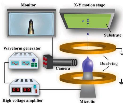
Fig. 11. Schematic diagram of DEF EJ technique. Reproduced from ref. 55 with permission from John Wiley and Sons, copyright 2023.
