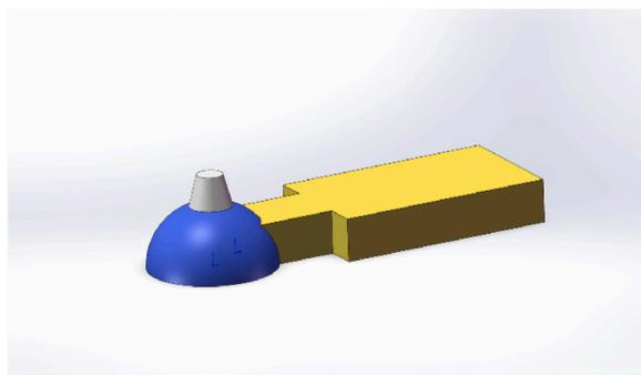
Fig. 7. Structure diagram of hemispherical cavity thermal inkjet printhead.
