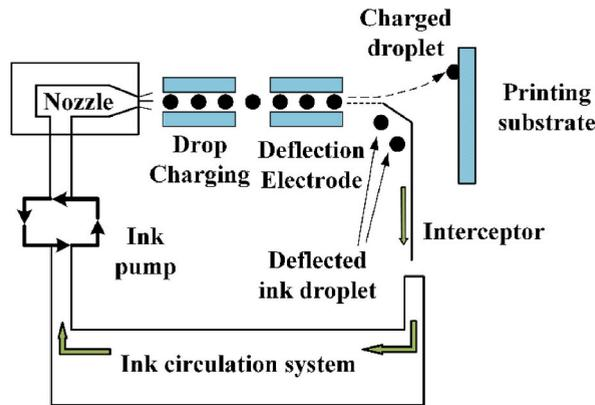
Fig. 2. Continuous inkjet technology principle and structure diagram.
