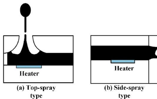
Fig. 5. Two types of thermal bubble structures: (a) top-jet printing (b) side-jet printing.
