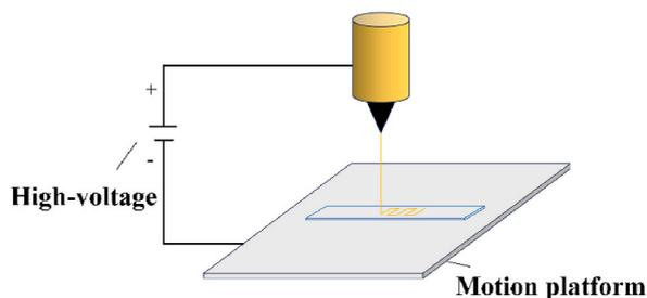
Fig. 6. Electric fluid principle structural diagram. Reproduced from ref. 106 with permission from Progress in Chemistry, copyright 2022.
