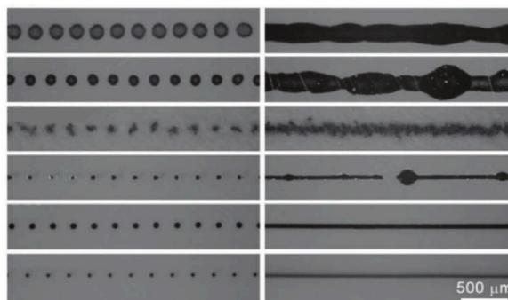
**Fig. 10.** Printing effects of AgNP ink on six different printing substrates: PEN, PET, copy paper, PI, PES, and photo paper. Reproduced from ref. 91 with permission from John Wiley and Sons, copyright 2023.
