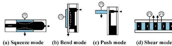
Fig. 4. When subjected to an electric field, piezoelectric crystals exhibit various deformation modes for ink extrusion: a) utilizing two piezoelectric crystals for ink extrusion, b) employing a single piece of piezoelectric crystal bending to expel ink, c) using a single piece of piezoelectric crystal for ink expulsion via pushing, d) employing multiple piezoelectric crystals for ink expulsion through shear deformation.
