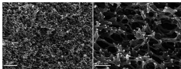
Fig. 4 Low- and high-resolution FE-SEM images for SnPOP.
