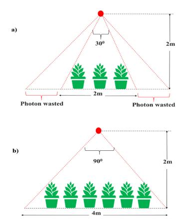
**Figure 1.** Impact of the PPF uniformity on the canopy photon capture efficiency. The canopy's photon capture efficiency (**a**) decreases as the lighting's fixture gets smaller and (**b**) increases as the installation of lighting gets more prominent. This concept and picture are modified [30].
