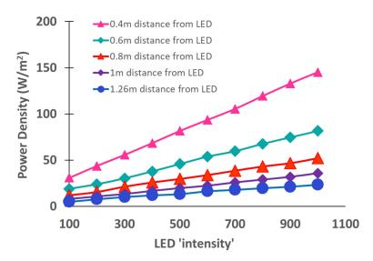
**Figure 2.** LED power density versus LED intensity for different distances from the LED source. The power density of the LED grows light is typically measured using a LaserCheck optical power meter to varying distances from the LED source.
