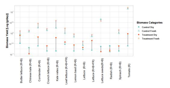
**Figure 4.** Effect of different LED illumination spectra on plant growth and development parameters, treatment fresh mass and treatment dry mass (with LED illumination), control fresh mass, and control dry mass (without LED illumination) for different vegetables and herbs grown in the growth chamber. Plants traits were log-transformed due to considerable variation in different treatments among species.
