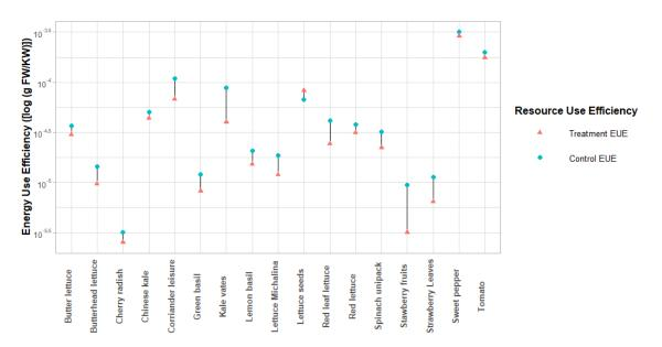
**Figure 5.** The energy use efficiencies (EUE) were calculated for vegetables and herbs grown in growth chambers, with (treatment) and without LED illumination (control) [15,44,57,84,109–111,119–121].
