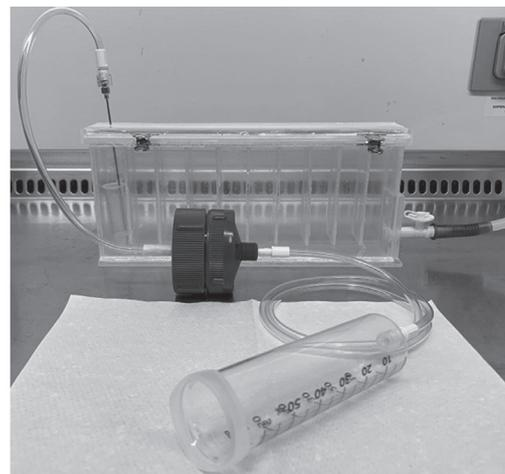
**Figure 1.** Sampling system for surgical smoke. Schematic and photograph of the sampling system.
