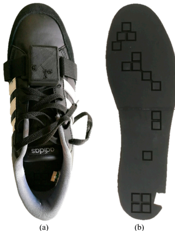
Figure 1. Prototype of pressure-sensitive insoles. (a) Shoes endowed with pressure-sensitive insoles. (b) Silicone cover.
