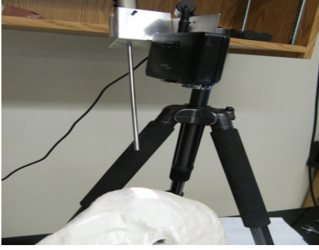
FIGURE 1: Experimental setup for stereo endoscope and liver phantom.
