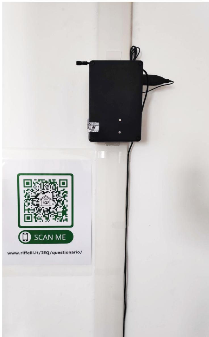
**Figure 9.** Wireless IEQ logger: system installation in the classroom.
