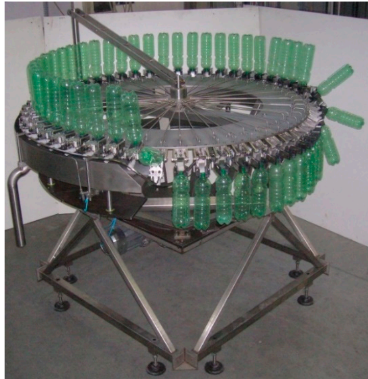
Figure 2. Bottle sterilizer machine with the base developed in [21]. External protection is not present in order to display the base.
