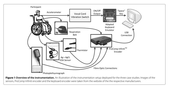
participant, a piezoelectric girth sensor (Thought Technology SA9311M) was secured thoracically over clothing but under the wheelchair restraints, in order to record respiratory waveforms.
