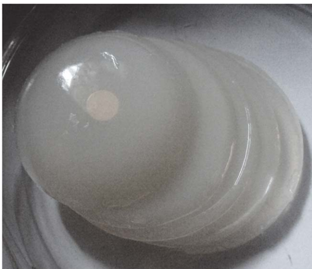
Figure 6. Breast phantom composed by five layers with the magnetic disk fixed at the first layer.
