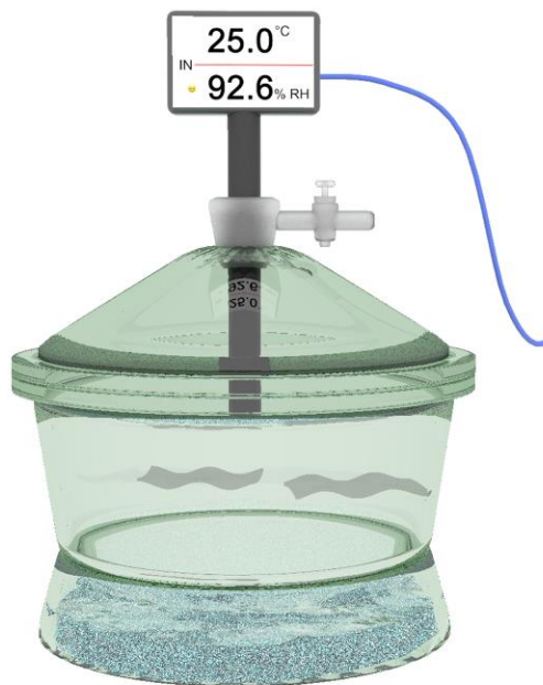
Figure S13. Schematic illustration of the device for measuring the moisture uptake of the separators, related to Figure 3C.
