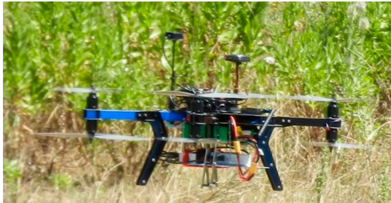
Figure 9. Customized X8+ by 3D Robotics used as flying deputy.
