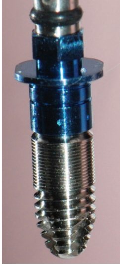
FIGURE 1: Experimental implant device: screw-shaped titanium implant packaged with fixture mount. The diameter and length of implant were 3.75 mm and 10 mm, respectively.
